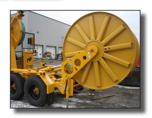
The BWPT45-1H/SL is a trailer mounted, self-loading puller / tensioner suitable for new construction and reconductoring construction. This unit is capable of pulling or tensioning single conductor.
